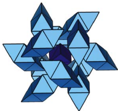
Figure 9 A tiling ( not natural) for fcc that has one kind of vertex, one kind of edge, one kind of face and one kind of tile. Note that pairs of tiles have at most one face in common. The symmetry is Pa\bar{3} .
