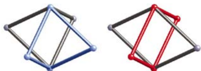
Figure 8 Skeletons of tiles for the bcc net. Left: a face ring (an essential 4-ring) is shown in blue. Right: an inessential 4-ring (not a face ring) is shown in red.
